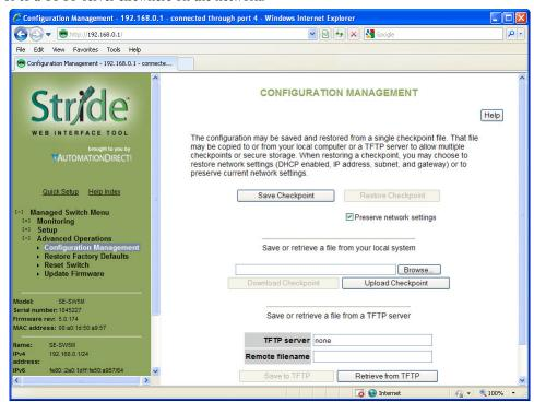
**Save Checkpoint:** Saves a checkpoint configuration in the switch, which may be used later to revert back to the current state if changes lead to an undesirable configuration.
