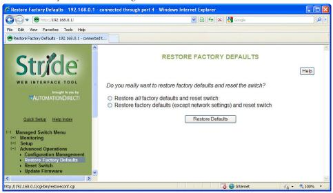
You can optionally choose to maintain the IP address configuration of the switch in order to more easily reconnect to the switch for configuration after resetting the defaults.
