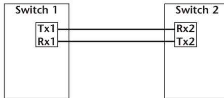
The fiber cable loss (LF) plus attenuator loss (LR) should be greater than the transmit power (TX) minus the receive power (RX).
