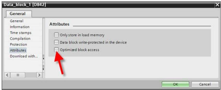
Use the Offset column of the Data Block as the byte address for StrideLinx. Even though the DB is defined as “Int” the offset is still byte not word.
