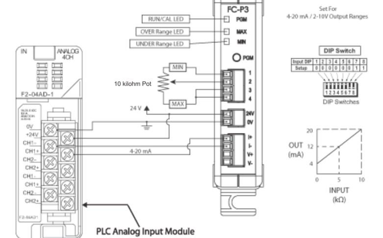
**CAUTION:** If current output (I+ / I-) and Voltage output (V+ / V-) are both connected to loads and/or the "I+" terminal to the "V-" terminal, product damage may occur.
