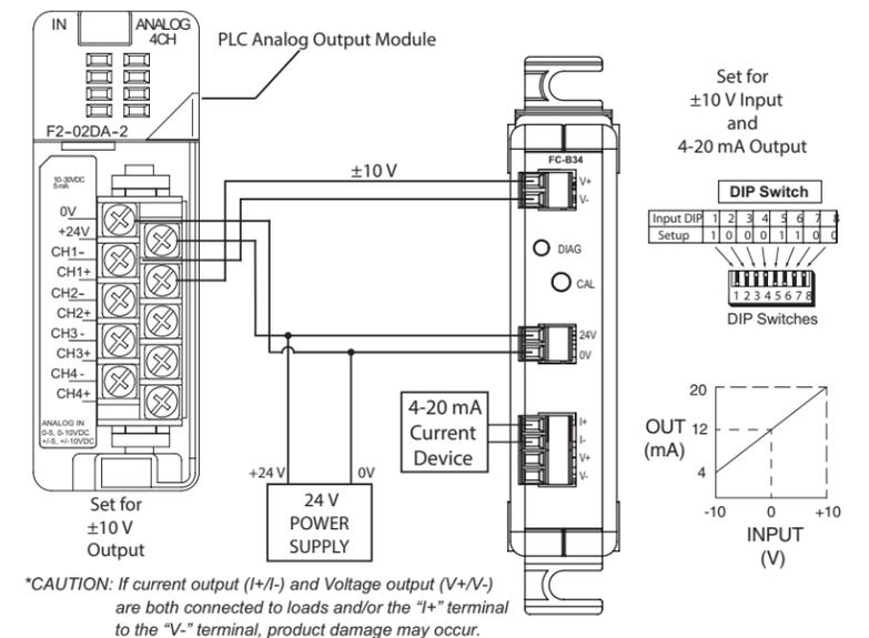
**\*CAUTION:** If current output (I+ / I-) and Voltage output (V+ / V-) are both connected to loads and/or the "I+" terminal to the "V-" terminal, product damage may occur.
