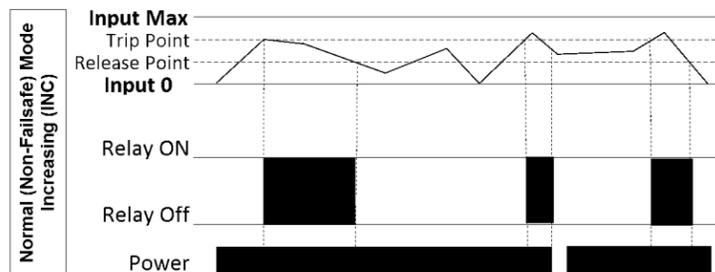
Normal (Non-failsafe) Mode [DIP Switch 6 OFF]
