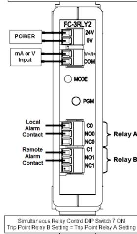
Normal (Non-failsafe) Mode [DIP Switch 6 OFF]
