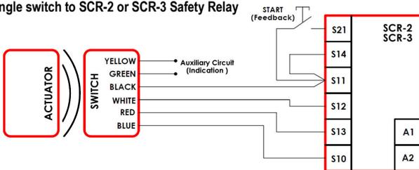
**Single switch to SCR-21-I or SCR-31-I Safety Relay (Viper range)**
