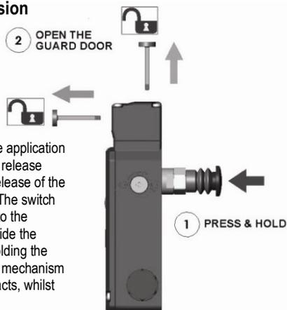
Where the Risk Assessment for the application permits, a non latching emergency release version (KLM-RR) enables quick release of the switch lock in case of emergency. The switch can be mounted such that access to the release button is available from inside the active guard area. Pressing and holding the release button will release the lock mechanism and open the lock monitoring contacts, whilst the guard can be pushed open.
