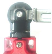
4. When mounting to the guard door, align and fix the switch body to the frame of the door using 2 x M4 mounting bolts tightened at 1.5Nm. Fix a Steel Actuator pin (diameter 5mm max.) to the frame of the guard ensuring that the full required opening position of the door can be achieved.
