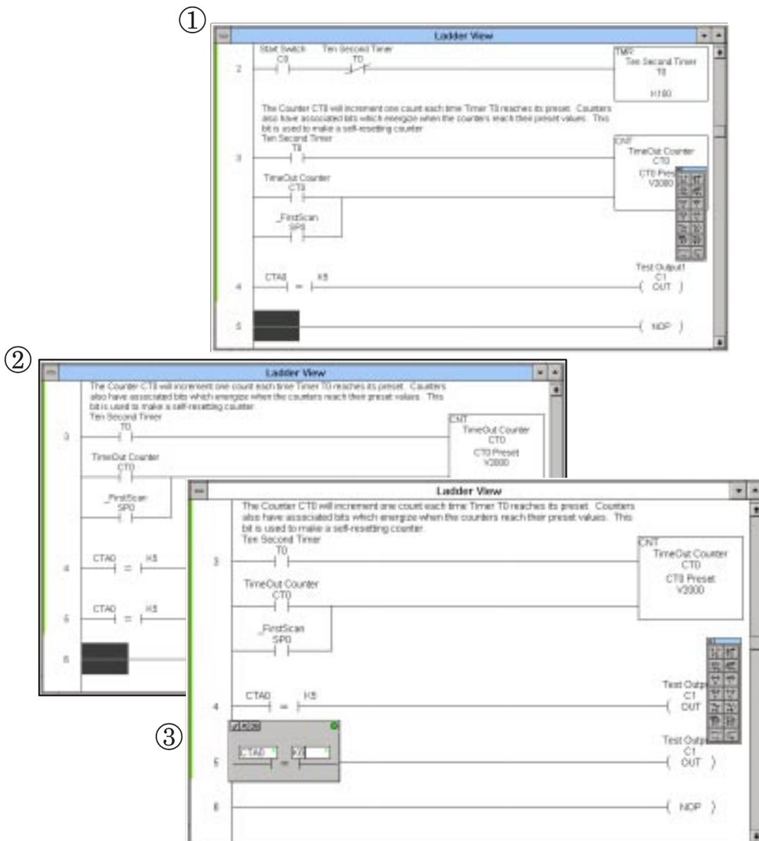
Next, move the cursor to the end of the pasted rung. With the cursor over the **C1** output element, double click with your mouse. This opens the window for editing the output coil. Change it to **C2**.
