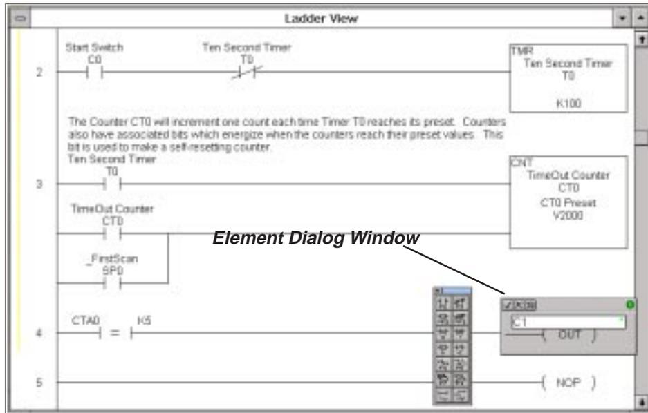
You can now enter the nickname **“Test Output1”** for **C1**, using the same procedure used earlier. Press the key combination **CTRL + D** to bring up the **Documentation Editor** and enter **“Test Output1”** into the **Nickname** window.
