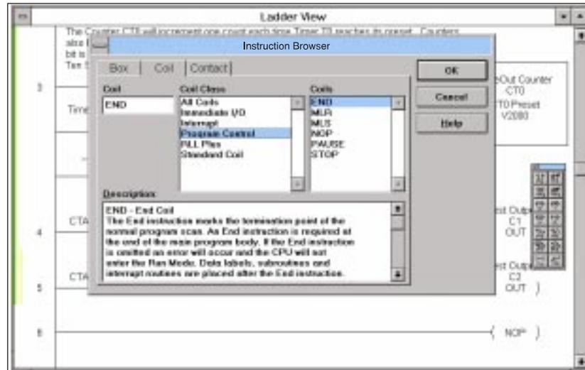
Click on **OK** when you are finished. With the final rung showing the **END** statement, you have now completed the program. Press **F8** to accept the rungs. Finally, click on the **Save to Disk** icon of the toolbar. You are now ready to connect and communicate with your PLC. Move to the next page and see how to download the program to the PLCs memory and test it.
