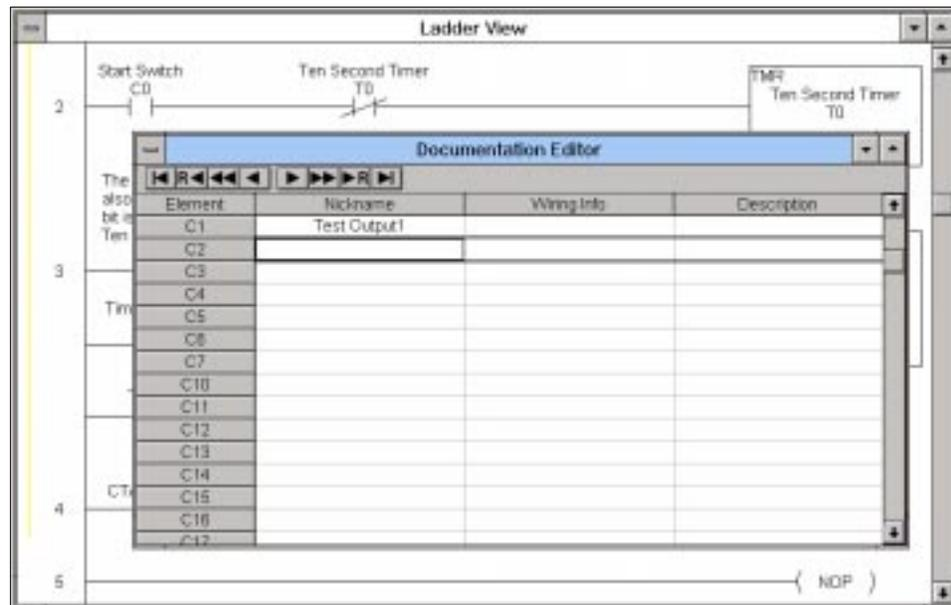
Close the **Documentation Editor** and return to the rung. Notice the Nickname **Test Output1** is now above the element. You are now finished with these rungs. **Accept** them by using the hot key **F8** or by selecting **Edit/Accept** from the upper menu bar.
