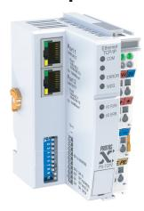
The PX-TCP2 Modbus TCP Server Bus Coupler allows connection of up to 64 terminals in a Modbus TCP network. The PX-TCP2 communicates using high-level Modbus commands and automatically assigns Modbus addresses for inputs and outputs. The maximum amount of data is 512 bytes of input data and 512 bytes of output data, with up to 512 inputs, 512 outputs, and 128 analog inputs or outputs.
