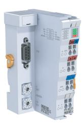
The PX-MOD Modbus RTU/ASCII Slave Bus Coupler allows connection of up to 64 terminals per assembly, 255 terminals total, in a Modbus RTU/ASCII serial network. The PX-MOD communicates using high-level Modbus commands and automatically assigns Modbus addresses for inputs and outputs. The maximum amount of data is 512 bytes of input data and 512 bytes of output data, with up to 1020 inputs, 1020 outputs, 256 analog inputs and 256 analog outputs, when using bus expansion.
