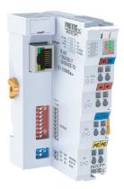
The PX-EIP1 consists of one RJ45 Ethernet 10/100 Base T port for connection to an Ethernet client. The PX-EIP1 performs as a EtherNet/IP server in an EtherNet/IP network. Communication to the client is via an RJ45 Ethernet port. The maximum distance from client to the PX-EIP1 is 330 feet (100 meters) using 24AWG shielded, twisted pair Cat5e cable. The PX-EIP1 Bus Coupler supports up to 64 terminals per assembly, 255 terminals with Bus Expansion Couplers.
