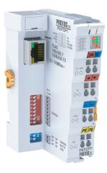
The PX-TCP1 Modbus TCP Server Bus Coupler allows connection of up to 64 terminals per assembly, 255 terminals total, in a Modbus TCP network. The PX-TCP1 communicates using high-level Modbus commands and automatically assigns Modbus addresses for inputs and outputs. The maximum amount of data is 512 bytes of input data and 512 bytes of output data, with up to 1020 inputs, 1020 outputs, and 128 analog inputs or outputs, when using bus expansion.
