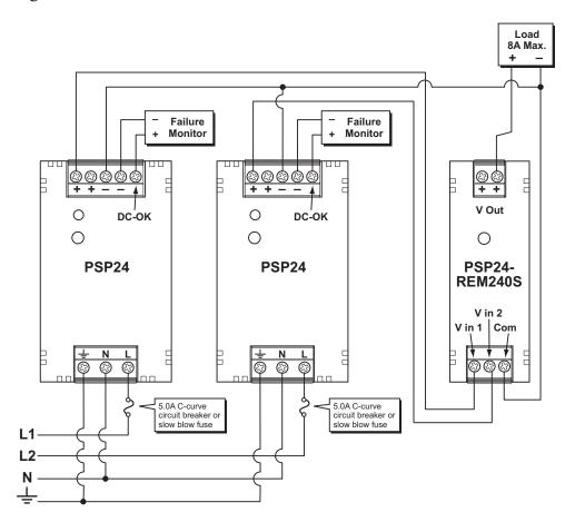
Recommendations for redundant PSP Series power supply applications:
