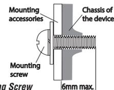
**Figure 4 - Mounting Screw**
