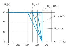
Note: Max. ambient operating temperature when wired for 4-20 mA output.
