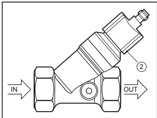
▶ Insert the unit into the pipe according to the direction of flow (arrow) and tighten.
