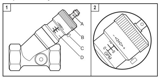
A: LED; B: setting dial; C: lock screw; D: setting scale
