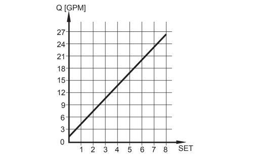
The diagram shows the typical course of the measurement curves for water at 20 °C.
