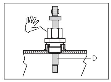
➤ Tighten the coupling nut manually and mark its position with a line (E).
