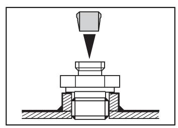
► Attach the coupling nut and insert the sensor (D).
