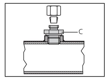
► Grease all parts of the adapter: coupling nut (A), ferrule (B), thread and cone of the fitting (C).
