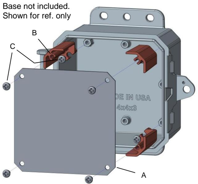
Position the Faceplate supports (B) (x4) flush against the inside wall of the Base and secure with #8-18 X 3/8" Pan Head Screws (C) (x4) into the hexagonal boss, as shown. Position the Faceplate panel (A) over the supports and secure with #8-18 X 3/8" Pan Head Screws (C) (x4) into the supports (B). Torque to 8-10 in-lbs., using Philips head #2 screwdriver.
