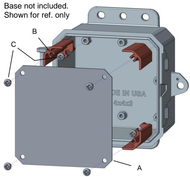
Position the Faceplate supports (B) (x4) flush against the inside wall of the Base and secure with #8-18 X 3/8" Pan Head Screws (C) (x4) into the hexagonal boss, as shown. Position the Faceplate panel (A) over the supports and secure with #8-18 X 3/8" Pan Head Screws (C) (x4) into the supports (B). Torque to 8-10 in-lbs., using Philips head #2 screwdriver.
