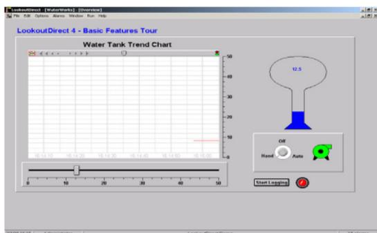
From this menu bar, select **Edit > Edit Mode** to set the screen to allow editing. The screen can also be toggled between **Edit** and **Run** by pressing CTRL - Space at the same time.
