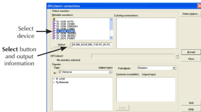
From the top left list, click on the device with the slot number and output point you want to use for your sample project. The output point will be highlighted. Now click on the **Select** button. The information for the output point will be displayed next to the **Select** button.
