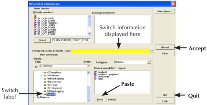
Once the switch reference text is shown on the address line, click on the **Accept** button to accept the output point and switch selections. Clicking on **Quit** will close the **OPC Client Connections** window.
