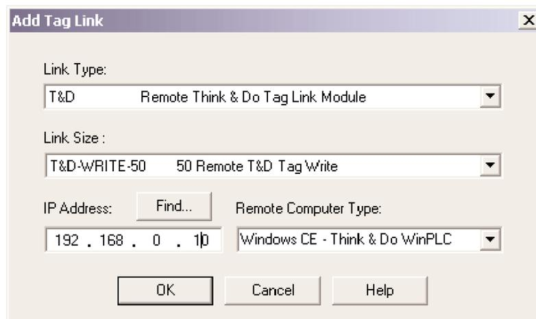
Select **T&D-WRITE-50 50 Remote T&D Tag Write** for the Link Size.
