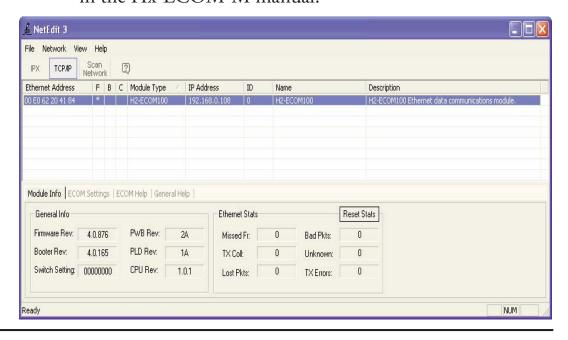
To use DataWorx, a connection must be established between the PC and the DirectLogic PLC. This connection will use the Ethernet network card in the PC to connect to an ECOM module in your PLC.
