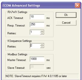
• ACK Timeout sets the time limit for receiving the acknowledge (ACK) response to an RX or WX instruction. The ECOM sends a message across the LAN. The acknowledge response comes back directly from the ECOM module receiving the transmission. ACK Timeout sets the maximum elapsed time in milliseconds for transmission and acknowledgement from ECOM to DataWorx across the LAN. It is not dependent on the PLC scan time.
