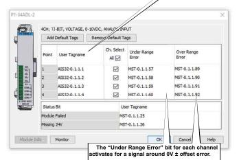
The "Over Range Error" bit for each channel activates for a signal around 10V ± gain error.
