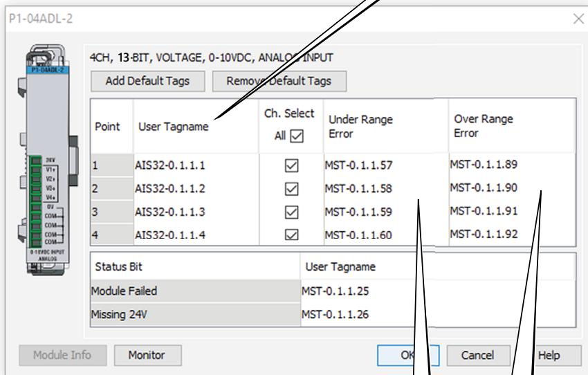
The “Under Range Error” bit for each channel activates for a signal around 0V,  $\pm$  offset error.
