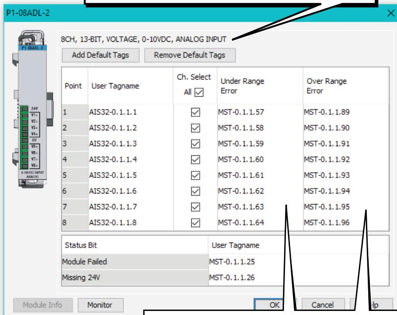
The “Under Range Error” bit for each channel activates for a signal around 0V,  $\pm$  offset error.
