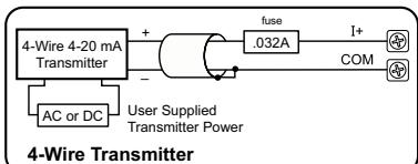
Note: Do not connect both ends of shield.
