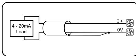
Note: Shield is connected to common at the source device.
