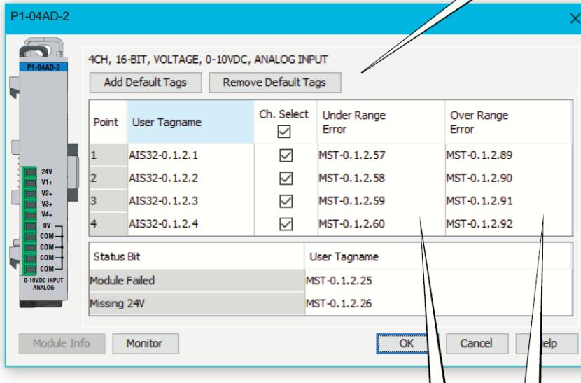
The “Under Range Error” bit for each channel activates for a signal around  $0V \pm$  offset error.
