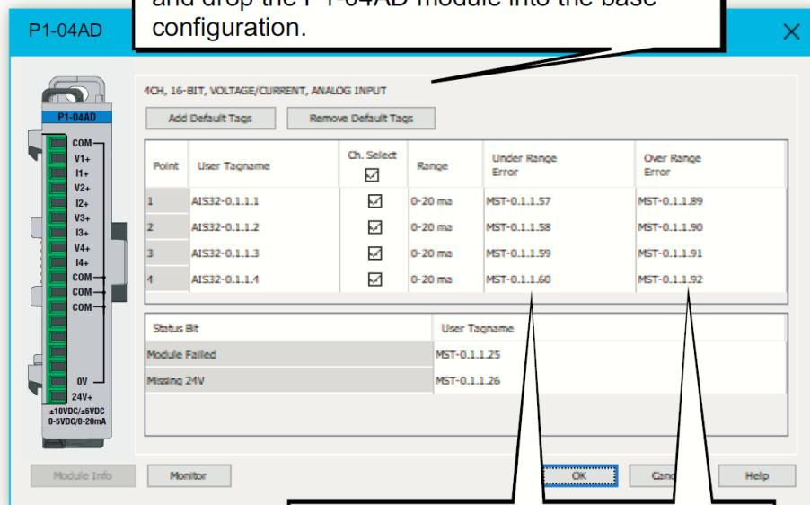
The “Under Range Error” bit for each channel activates for a signal around  $0\text{mA} \pm \text{offset error}$ .
