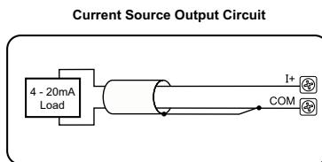
Note: Shield is connected to common at the source device.
