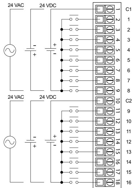
Equivalent Input Circuit
