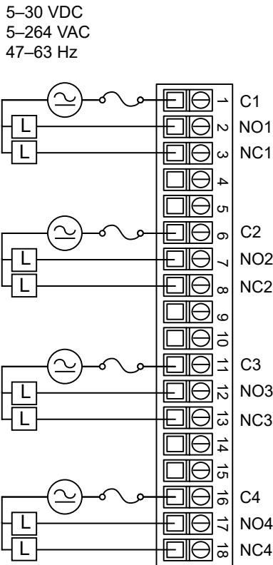
**Equivalent Output Circuit**
