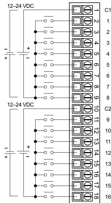
Equivalent Input Circuit
