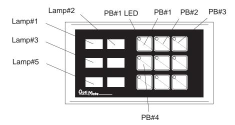
If you look at the pre-configured OP-WINEDIT program you loaded into the OP-panel earlier, notice that pushbuttons PB#1, PB#2, and PB#4 are set for momentary operation and that PB#5 through PB#9 are set for alternate (toggle) operation. Also, the Force Option and LED Separation features are both activated (see Configuration section for configuration details).
