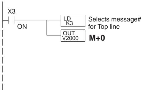
In this example, if the PLC's input signal X3 is ON, the 16 bit integer (K3) value is placed in Word register V2000 (M+0), selecting message #3 to be displayed on the top line.
