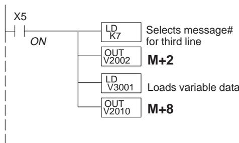
In this example, if the PLC's X5 input signal is ON, the 16 bit integer (K7) value is placed in Word register V2002 (M+2) requesting message #7 to be displayed on the third line. The data value in register V3001 (let's say 1101) is moved into V2010 (M+8), which is embedded in the third line message. The third line data value will update as long as X5 is enabled (ON).
