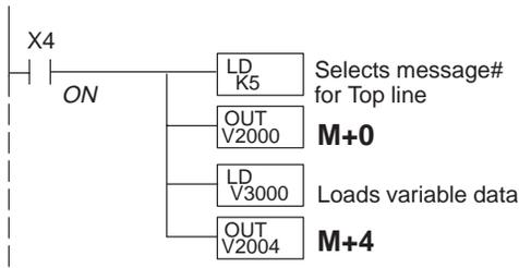
In this example, if the PLC's input signal X4 is ON, the 16 bit integer (K5) value is placed in Word register V2000 (M+0) selecting message #5 to be displayed on the top line. The data value in register V3000 (let's say 1100) is moved into V2004 (M+4), which is embedded in the top line message. The top line data value will update as long as X4 is enabled (ON).
