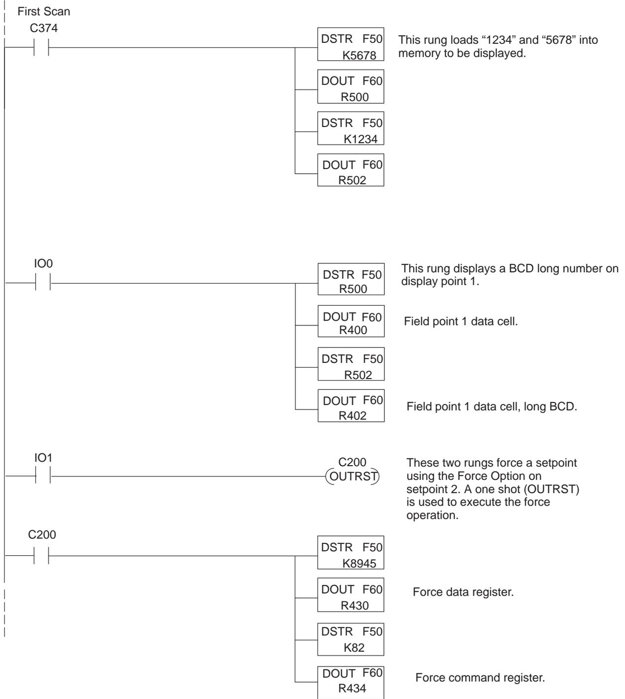
**Reading a Setpoint** The OP-414 continuously updates the registers of all setpoints with each setpoint's current value. To read a setpoint, simply access the register(s) that correspond to each setpoint. The data can be copied to another register for manipulation or it can be accessed in its field point register(s).
