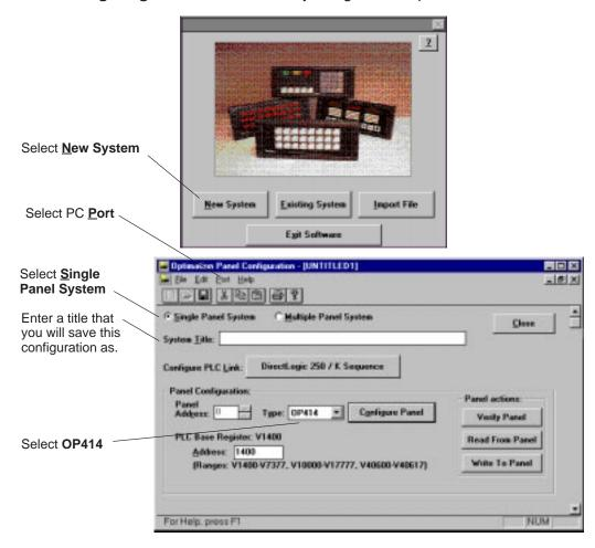
Step 5 Select Configure PLC Link – Here is where you define protocol items such as PLC address, baud rate and parity. Enter the appropriate parameters for your PLC. The following table provides the necessary information for most PLC Direct controllers. For other PLC families, reference that product's user manual to determine the port communications capabilities.
