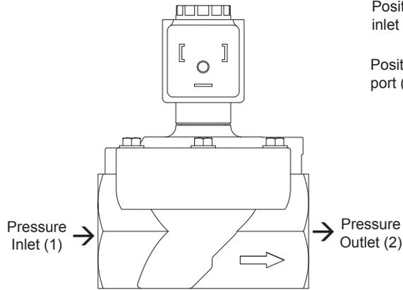
Position 1) Coil De-energized. Pressure inlet port (1) is closed to outlet port (2).
