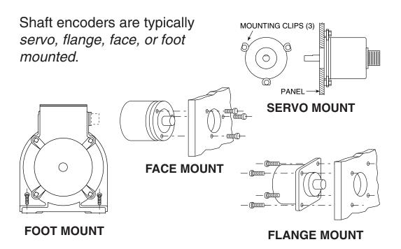
Because shaft encoders have no flexture, mechanically coupling one to a machine requires important consideration. Backlash or modulation in the coupling can cause errors in position indication. Rigid attachment of the shaft may cause bearing failure. Therefore, a *flexible coupling*, which compensates for misalignment between the encoder shaft and the machine, must be used.
