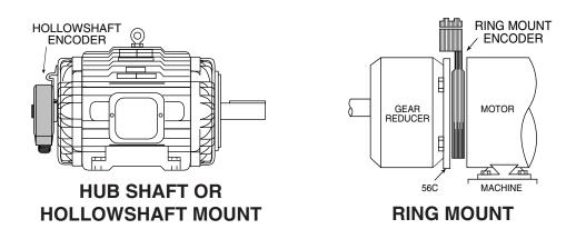
A hub shaft or hollowshaft encoder should be mounted so that its shaft receptacle is in as close as possible alignment with the axis of the driving machine or motor shaft. Clamp or set screws should then be tightened to secure the encoder. NOTE: Do not defeat or restrict the flexure. This causes failure of the encoder or driving shaft bearings.
