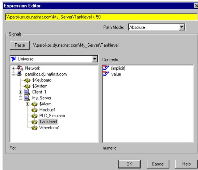
You can then connect this logical result to a PLC or RTU to control the fill valve so that the valve opens when the tank level drops below 50 and closes when the tank level rises above 50. Notice, however, that this method can cause the valve to fluctuate between open and closed too often if the tank level hovers around 50.
