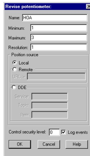
In the following **Create expression** dialog box, a three-position switch is created with the Pot object class, where 1=Hand, 2=Off, and 3=Auto.
