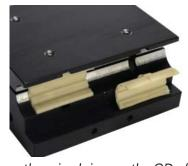
Make sure the raised ring on the OD of each liner is constrained in its groove on the carriage. Also make sure the raised cylindrical nub at the middle of each liner is seated in its circular pocket located at the seam between the top and bottom carriage sections.
