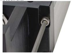
26) Move the carriage to the center of the system and fasten the new lead screw nut to the carriage with the original lead screw nut mounting screws.
