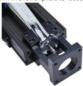
5) Use a 3/32-in hex key to remove the idler end mount screws. Pull the mount off the end of the lead screw.
