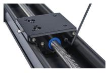
11) Use retaining ring pliers to remove the retaining ring in the idler and mount. Remove and discard the bearing and the retaining ring.
