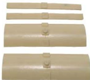
18) Lay the carriage on its side and insert one of the two larger slide bushings into the housing. You will feel a positive snap when it falls into correct placement. Now place the second large slide bushing into the carriage so that it snaps into place. A little grease on the back side of the bushings will help to hold it in place until the slide tube is engaged.
