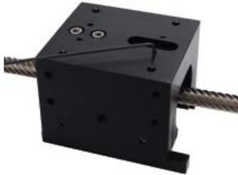
16) With a 1/16-in hex key, loosen the two side adjusting screws. Loosen one full turn each. Repeat for the other two side adjusting screws on the opposite side.
