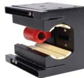
19) Carefully slide the carriage onto the slide tube while holding the slide bushings in place. Ensure that the lead screw drive nut portion of the carriage is away from the drive end of the screw to allow for easier engagement and proper nut positioning.
