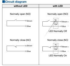
When using the switches with LED option, limit the current below 10mA.
