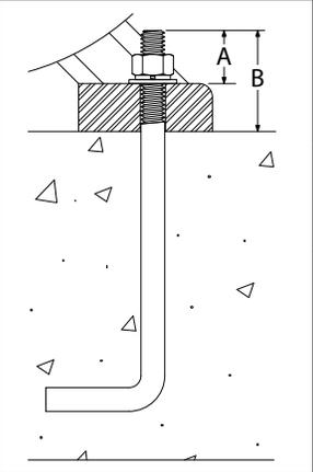
The diagram shows a cross-section of a motor being mounted to a surface. A bolt is used to secure the motor's base. Dimension 'A' is the length of the bolt's thread that is engaged in the motor's base. Dimension 'B' is the length of the bolt's shank that is embedded in the mounting surface. The diagram also shows the motor's base with mounting feet and a cross-section of the mounting surface with shims.
