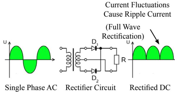
Form factor is the ratio of  $I_{rms}$  to  $I_{dc}$  and indicates how close the driving voltage is to pure DC. The form factor for a DC battery is 1.0. The higher the form factor is above 1.0, the more it deviates from pure DC. The Form Factor Table shows examples of commonly used voltages.
