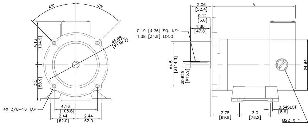
A = 8.0" [203.2] - 0.33 HP, 90VDC, 1800RPM
