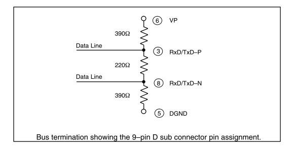
Communication speeds between 9.6 kbps and 12 Mbps are available. One unique baud rate is selected for all devices on the bus when the system is commissioned. The baud rate selected will depend upon the cable length.
