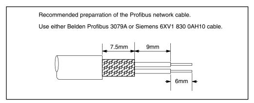
After preparing the cable, insert the green and the red conductors in the appropriate screw terminals of the bus connector.
