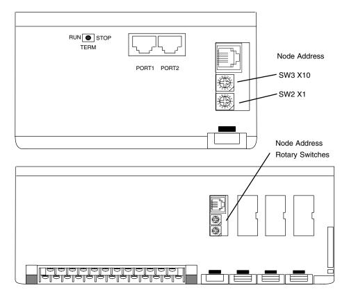
Remove the cover associated with the option slot where the H0–PSCM is installed in the DL06. Once the access cover is removed, use a small, flat, screwdriver to set the Node Address to an available address, from 3–125. Node Address 0 is normally reserved for the Profibus network master. Note that SW3 sets the tens and SW2 sets the units.
