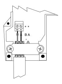
Termination showing the cable connection to points A (Red) and B (Green).
