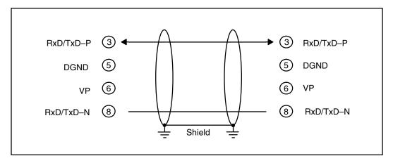
The two wires are usually color coded. Typically red and green are used. Red is used for the **B** Transmit/Receive line and Green for the **A** transmit/receive line. It is important to keep A and B line consistent throughout the network to avoid improper operation. *This is the most common connection mistake in the field.*
