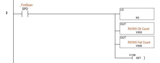
Once the ECRX and ECWX IBoxes are enabled, the ECOM100 IBox will automatically sequence them, no manual control of the port busy bits is required.
