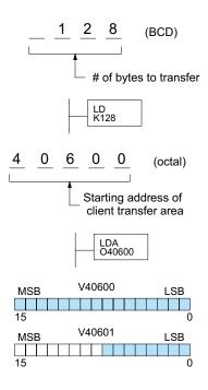
For an RX instruction, the CPU reads the number of bytes previously specified from the server, placing the received data into its memory area beginning at the LDA address specified.
