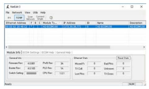
In the graphic above, double-click the ECOM100 desired. This will pull up the following **General Settings** box. Here, you can assign the IP address and subnet mask for his network. The Modbus slaves will need to have compatible settings of course. When finished , click OK to go back to NetEdit main screen.
