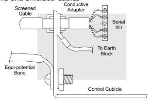
Good quality 24 AWG minimum twisted-pair shielded cables, with overall foil and braid shields are recommended for analog cabling and communications cabling outside of the PLC enclosure. To date it has been a common practice to only provide an earth ground for one end of the cable shield in order to minimize the risk of noise caused by earth ground loop currents between apparatus. The procedure of only grounding one end, which primarily originated as
