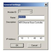
Assign a module ID: The module ID is only required when the master's address mode is set to Module ID.
