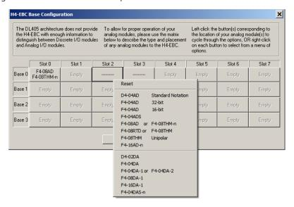
Once the correct part numbers are chosen for each of your analog modules, click the OK button to save the configuration into flash memory onboard the module. Leave the symbol "-----" wherever you have a digital module.
