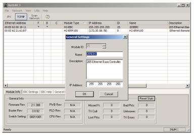
Module IDs must be unique for each module, but they do not have to be in sequence. The DIP switches must all be set to zero to enable any software to change the Module ID. If not set to zero then the Module ID will be read only.
