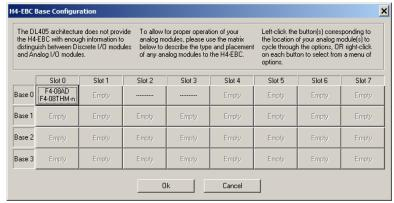
The default symbol "------" appears on the configuration screen where digital or analog modules are present. For digital modules, you do not need to make any changes. The H4–EBC recognizes the digital modules and is self-configuring for the digital modules.
