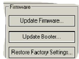
Clicking on the either of the Update buttons opens the appropriate EBC folder within the Images folder, which is created during the install of NetEdit3. The Images folder is located in the same folder as NetEdit3.exe. Each module folder contains the module's firmware and boot loader files. The next section discusses keeping the firmware files up to date.
