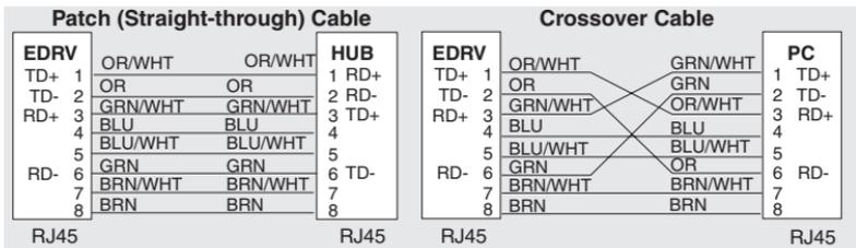
This diagram illustrates the standard wire positions in the RJ45 connector. We recommend all Ethernet 10/100Mbps cables to be Category 5, UTP cable.
