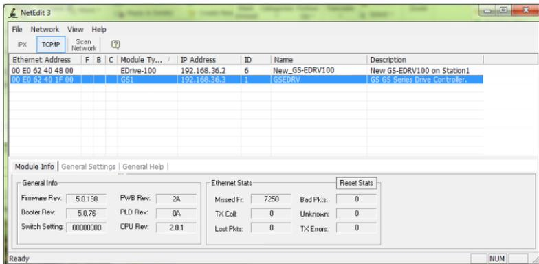
Double click on the desired GS-EDRV. A "General Settings" popup will display allowing you to configure the IP address of the module you have selected.
