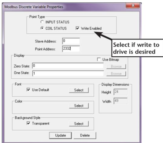
Once a read/write data object is created, double click on the object and a Write Modbus Variable popup will appear allowing the user to enter a new value for the selected parameter.
