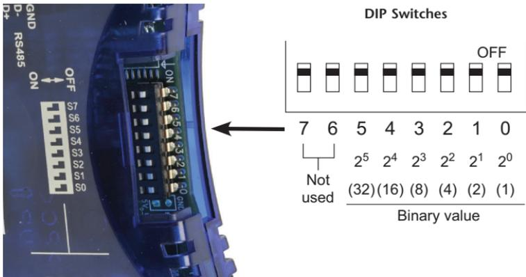
The ID equals the sum of the binary values of the slide switches set in the ON position. For example, if you set slide switches 1, 2, and 3 to the ON position, the ID will be 14. This is found by adding  $8+4+2=14$ . The maximum value you can set on the DIP switch is  $32+16+8+4+2+1=63$ . This is achieved by setting switches 0 through 5 to the ON position.
