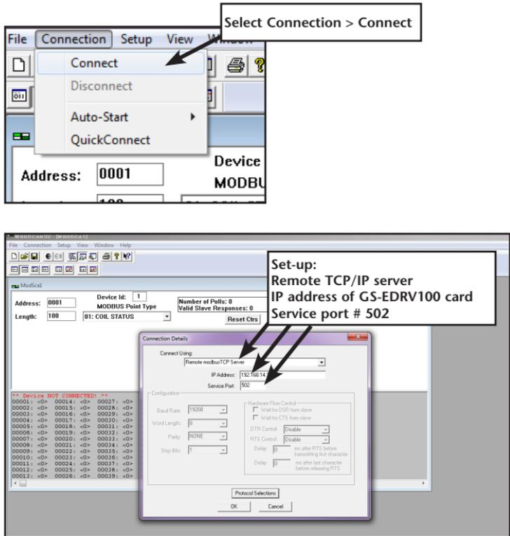
Once a connection to the interface has been established, select the drive parameters that you wish to monitor. See the table below for drive parameters and their modbus addresses.
