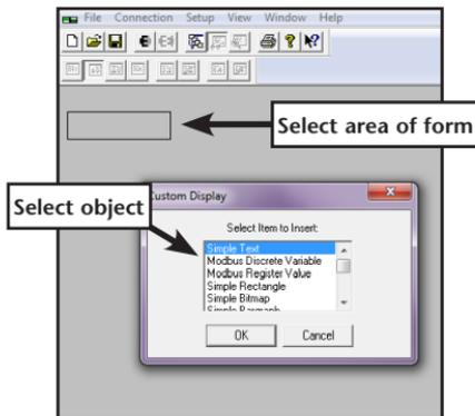
Select an object (text, charts, shapes or data) from the menu and ModScan will load the selection into the form. When creating data objects, such as Register and Discrete variables, selecting the Write Enabled checkbox (as seen on following page) will allow the user to write values out to the drive from this f
