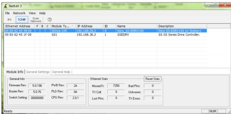
Double click on the desired GS-EDRV100. A “General Settings” popup will display allowing you to configure the IP address of the module you have selected.
