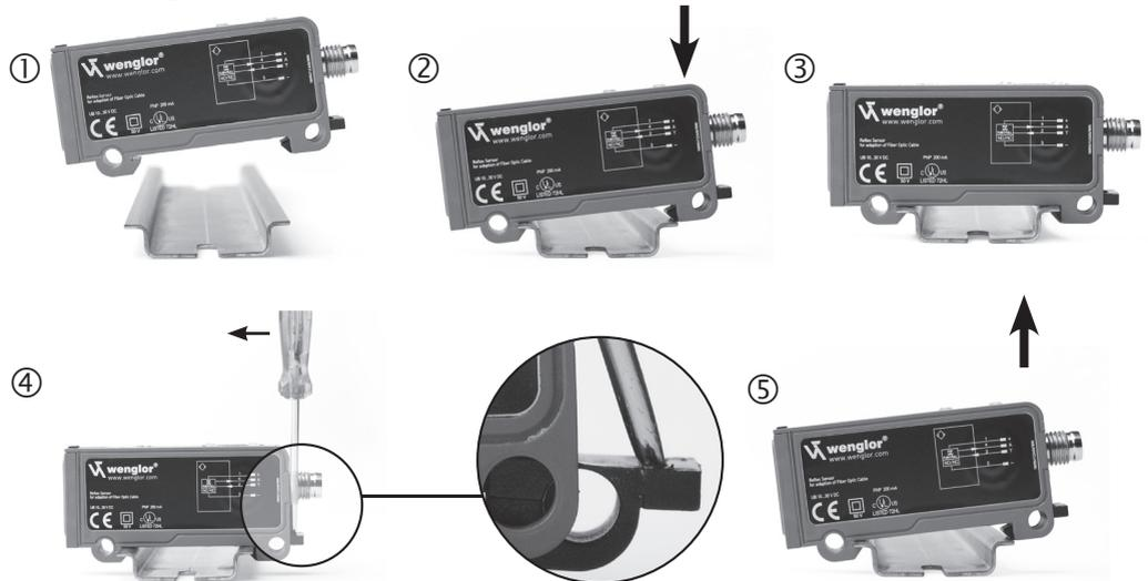
fig.1 Mounting of the Sensor to a DIN rail
