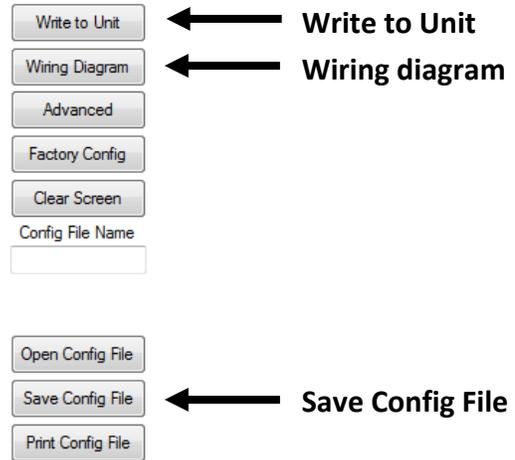
Next, use the file management features to save your configuration by clicking **“Save Config File”** and print your wiring diagram by clicking **“Wiring Diagram.”**
