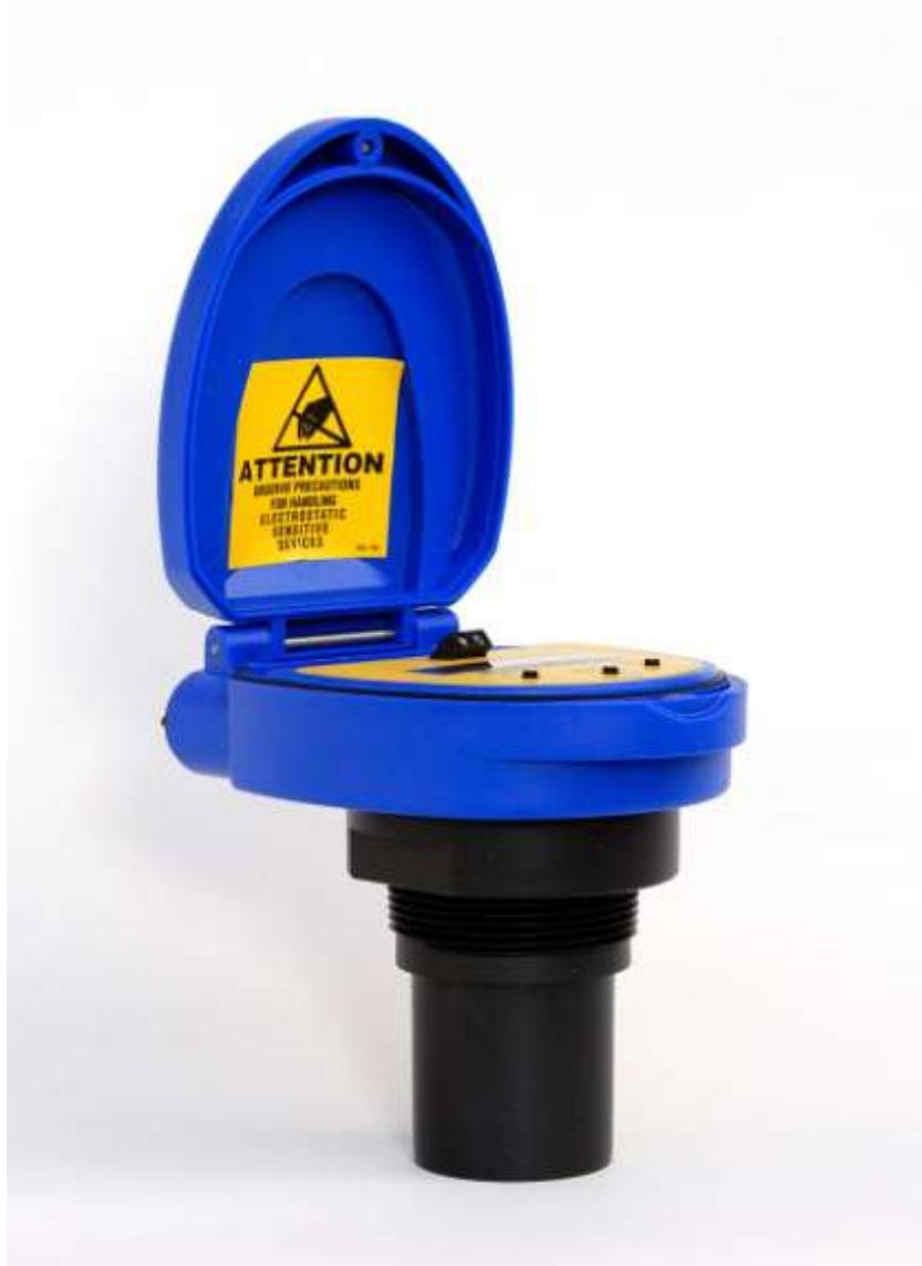
The EchoSpan® is a general-purpose ultrasonic level transmitter that provides a loop powered 4-20 mA output. The 4-20 mA output can be used to provide the proportional level of liquid in any tank or vessel. The signal can be connected to any device that accepts a loop powered 4-20 mA signal, such as a PLC, SCADA, DCS, display, controller, etc.
