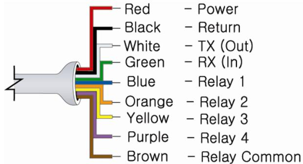
**Red** and **Black** leads are for connection to a 24 VDC power supply. The red and black wires can be extended more than 1000 feet using 22 gauge or larger wire, however do not extend the green and white wires.
