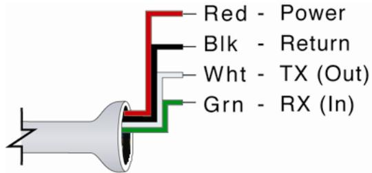
**Red** and **Black** leads are for connection to a 24 VDC power supply or to a 4-20 mA loop power source. The red and black wires can be extended more than 1000 feet using 22 gauge or larger wire, however do not extend the green and white wires.
