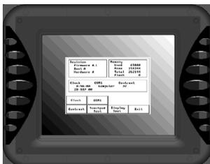
After the EZTouch Panel is powered up, you may enter the Setup Mode by simultaneously pressing the extreme upper left and lower left touch cells on the panel screen. The following screen is displayed. Information is displayed in the upper left hand corner about the current revision of the Firmware, Hardware, and Boot program. Also shown is RAM memory — Used, Free and Total, and Flash memory.
