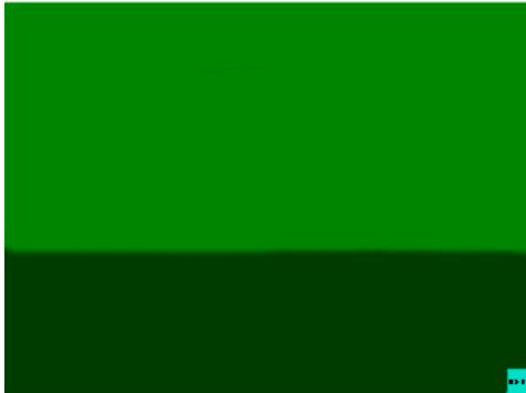
The Display Test button is primarily used for production testing at the factory. Bands of color scroll horizontally and vertically across the screen during this test. It is used to check the pixel quality of the display before shipping the unit.
