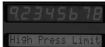
**Data Values** in messages can be of two types — Decimal and BCD. These two types can be in two different formats— with variable decimal point or without. Decimal point values can be in either variable or fixed position.
