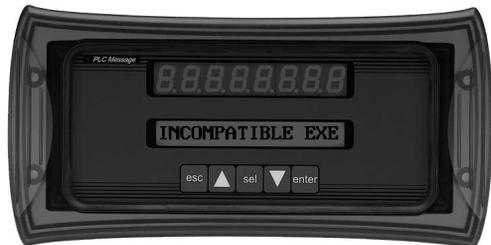
\* Because the EZText Set Point Display Panel LCD window display is limited to 16 characters, the message INCOMPATIBLE EXEC will display as INCOMPATIBLE EXE. (The "C" in EXEC exceeds the 16-character limit and will not display.)
